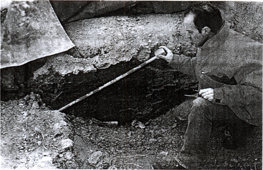
Figure 4: A portion of the surface of the reactivated Nojima Fault showing the relative movement between the fractured blocks.
